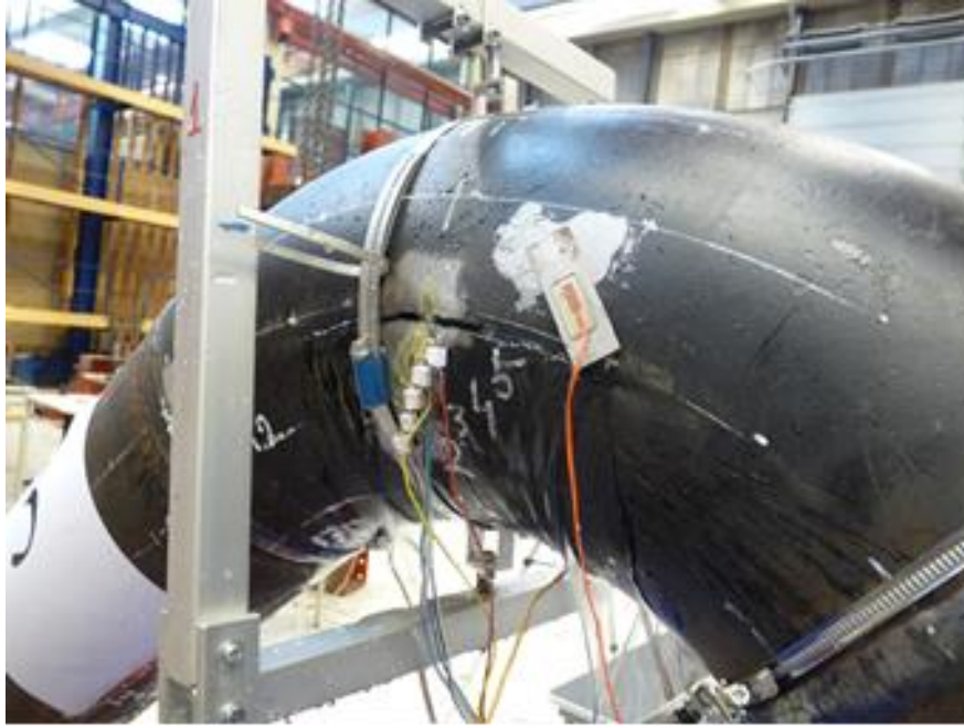
Figure 4. 6: Crack location at the elbow “flank”.
