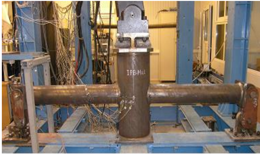
Figure 5.2: Test configuration for IPB loading.
