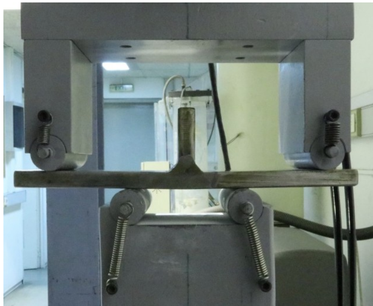
Figure 46. Experimental setup for welded T-joints.
