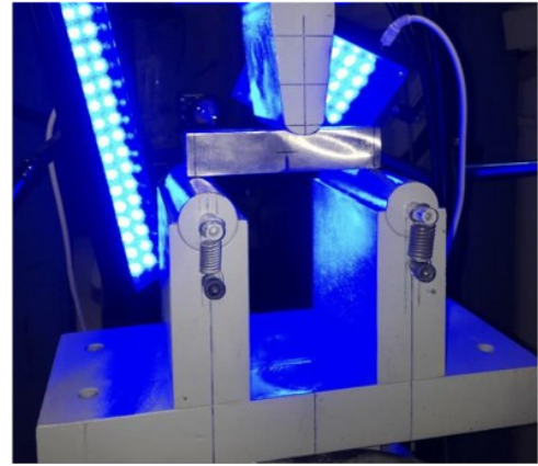
Figure 22. Schematic representation of CTOD specimen (a), and experimental CTOD test setup (b).
